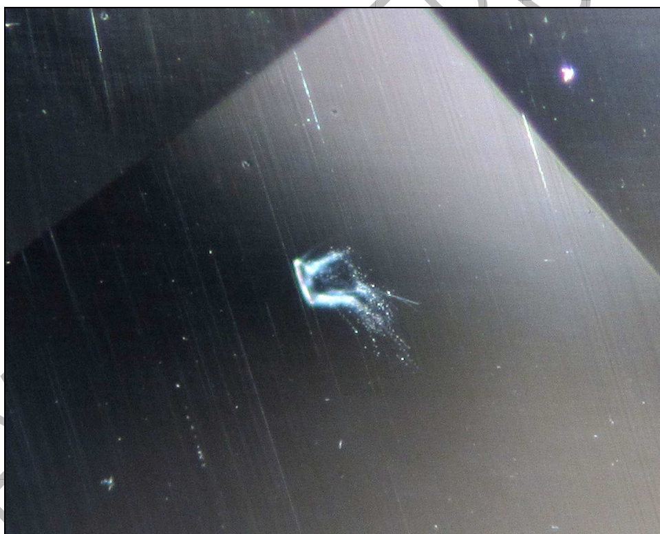
A phenakite crystal with "comet tail" due to growth blockage (dark field lighting 80x)
